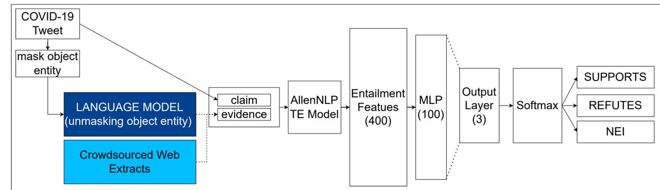
Figure 2: Full diagram of fact-checking pipeline. 'Evidence' is either generated by LM (dark blue) or taken from crowdsourced web extracts (light blue).
